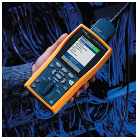
Certification tools take very precise measurements on parameters defined by the TIA and ISO standards. Documented results from a high-accuracy certification tool are the only means of meeting the requirements of manufacturers' warranties.
